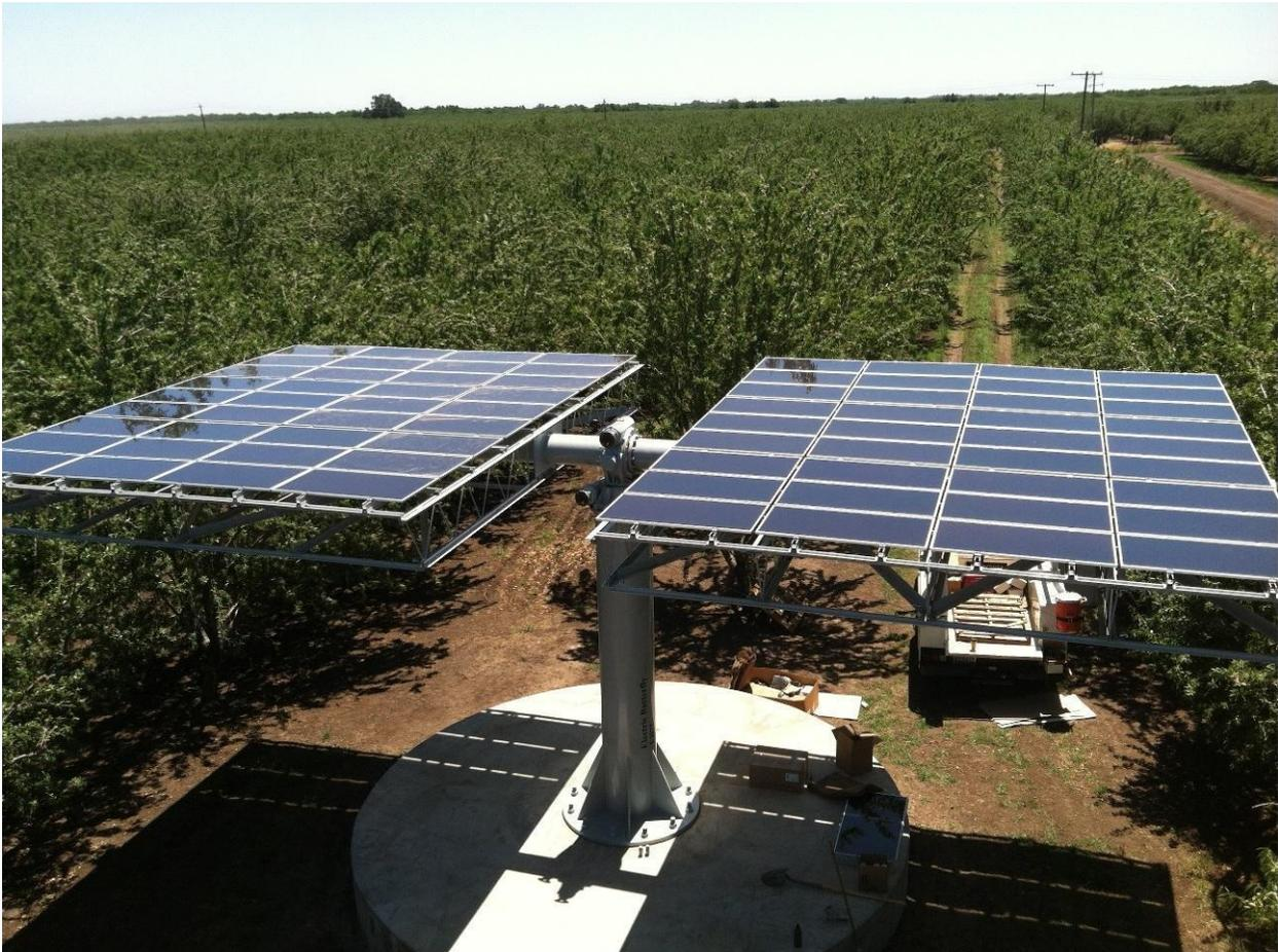
Pictured above is the USA made Electric Butterfly™, located on an almond orchard in Butte County, California. This is a robust two-axis tracker that can be installed in orchards, parking lots or other underutilized land spaces throughout California. The Electric Butterfly™ meets Category 5 earthquake requirements and Category 3 hurricane wind requirements in the stowed position.
